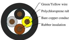
Polychloroprene rubber outer jacket Bare copper conductor
